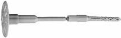
Dowel screw for flush or recessed mounting into insulation with long expansion area. Universally applicable to new and old buildings. Suitable for concrete, for solid, hollow and porous bricks, as well as for aerated concrete. Anchoring depth: 25 mm. Tolerance range  $\leq$  35 mm. ETA 12/0093. Use category: A/B/C/E. A Concrete/B Full stone/C Brick/E Aerated concrete. Thermal conductivity: I 10 dry  $<0,002$  W/mK. Shaft:  $\Phi$  8 mm – Retaining plate:  $\Phi$  60 mm.
