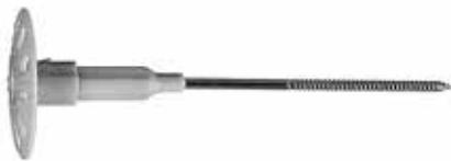
Insulation plate dowel with integrated thermally decoupled steel screw for mechanical fixing of thermal insulating panels on wooden substrates. Anchoring depth: 30-40 mm.
