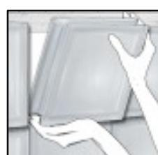
The vertical separation ARS-H19 will be dispensed with. Apply a reduced quantity of ReadySil silicone both in the last vertical separation and in the horizontal profile. Do not apply silicone to either the upper surface of the last block or the side of the same where the vertical separation had not already been placed.
